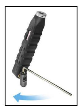
Select the test insert depending on stud diameter, push it on a torque wrench and fix it.
