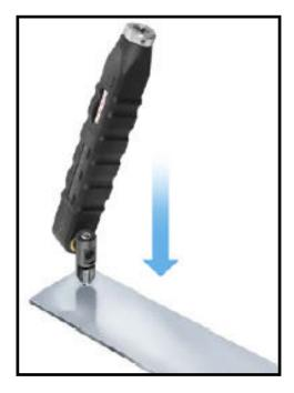
As shown in the figure, push the test device onto the stud. A torque is initiated with the torque wrench in a defined distance to the sheet surface. A bending strain of the weld results.
