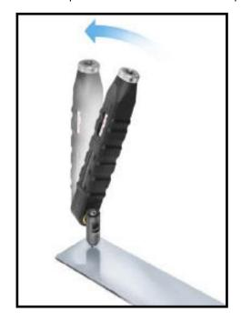
Move the test device forward/up until the device 'clicks' (attaining the nominal torque).
