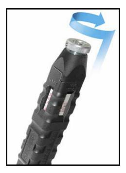
Depending on the test job, adjust the test torque of the torque wrench. Adjust the test torque in such a way that there is no permanent distortion of the welded parts.
