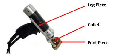
When the legs and foot piece are in place, insert the stud to be welded into the collet. Adjust the leg and foot piece by sliding it into position until approximately 1/8" of the stud protrudes from beyond the foot piece. Lock legs in place with the set screws.
