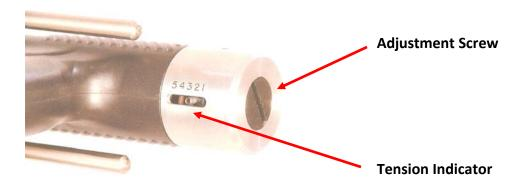
This spring pre-load adjustment is made by turning the screw insert in the back of the stud gun with a screwdriver. On the bottom of the back cap of the stud gun is the indicator numbered 1 thru 5, which will show you the tension setting during the adjustment.
