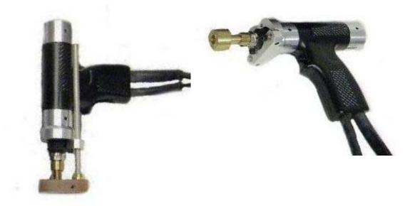
When removing the stud gun from the welded stud, always lift the stud gun vertically from the welded stud in order to maintain the proper tension of the collet. Spreading the collet when lifting the stud gun from the welded stud will shorten the life of the collet and will eventually create an undesirable weld.
