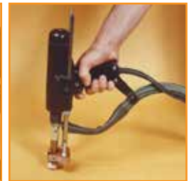
Position on the work piece and pull the trigger
