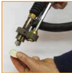
Load a ceramic arc shield (ferrule)
